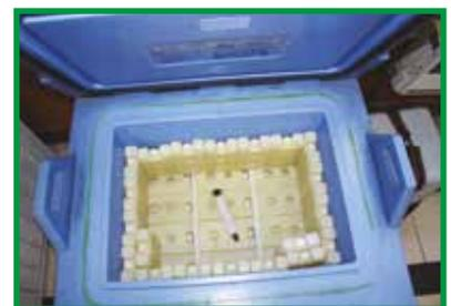
Cold box packed with icepacks and having a thermometer
